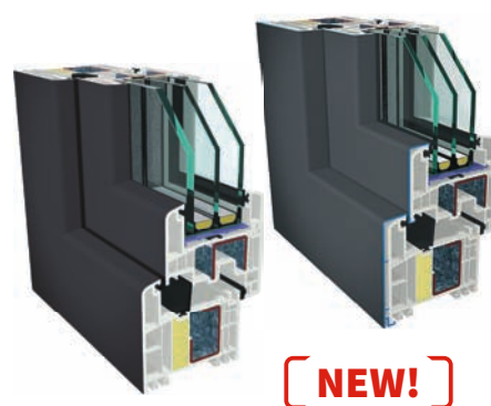
Futura / Futura Alu Modern PVC system. Construction depth: 83 mm. Foam insulated frame. Triple gasket system. Also available with aluminium cladding.
