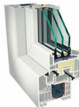
STV+IKD® Construction depth: 83 mm. Triple gasket system. Foam insulated sash (IKD). Special technique of glass adhesion (STV).
