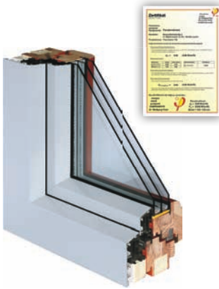
Alutrend Miratherm Construction depth of 126 mm, Uw from 0,70 W/m²K.
