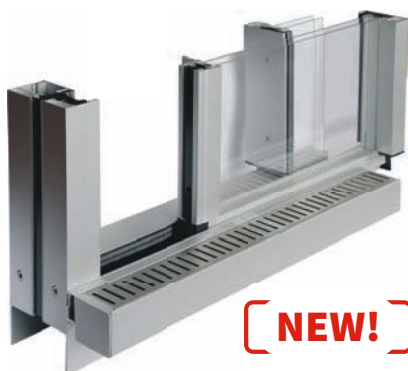
Artline / Artline XL High performance thermally insulated sliding door system with a slim sightline near the meeting stile (26 or 38 mm).
