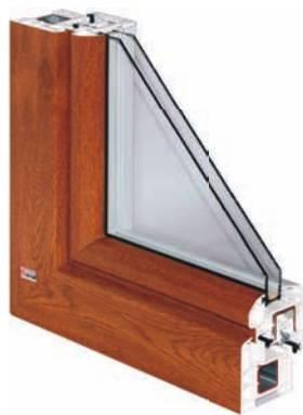
Comfort / XL - rounded 5/6 chamber system with additional central fin, construction depth: 74/83 mm. Rounded sash profile.
