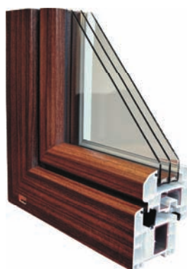
Kombisystem rounded 6 chamber system, construction depth: 83 mm. Rounded sash profile. Triple gasket system.
