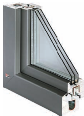
Comfort / Comfort XL 5/6 chamber system with additional central fin, construction depth: 74/83 mm.
