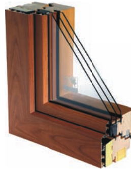
Ultratherm Basic Construction depth of 122 mm, Uw from 0,67 W/m²K.
