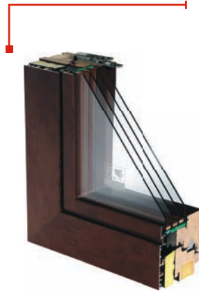
Ultratherm Ultima Construction depth of 125 mm, Uw from 0,69 W/m²K.
